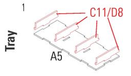
Required parts: **A5,A6,C8,C11**x2,**D8**x2
