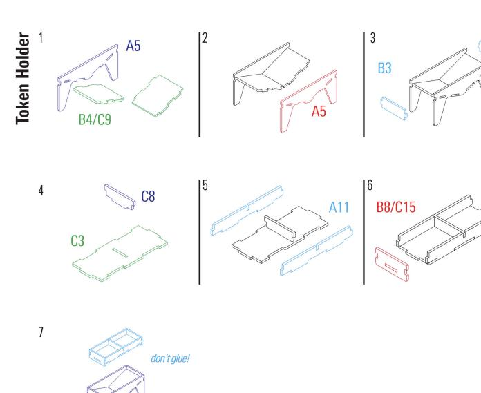
Required parts: **A5**x2, **B4**, **C9**, **B3**x2, **C3**, **C8**, **A11**x2, **B8**, **C15**
