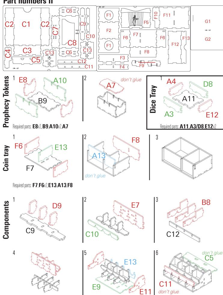
Required parts: C9, D9x3, C10, E7, C12, B8x3, E9, E13, E11x2, C11, C5,
