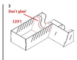
Required parts: C3, D1, D2, D3, E1, E2x2, F1x3, F3,
