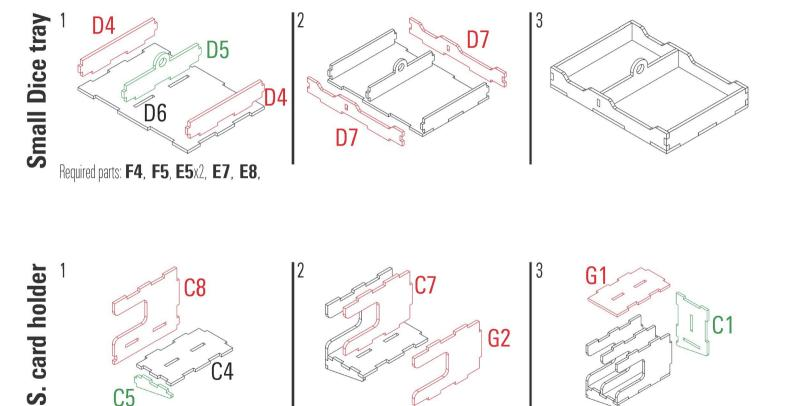
Required parts: C1x2,C4x2,C5x2,C7x2,C8x2,G1x2,G2x2
