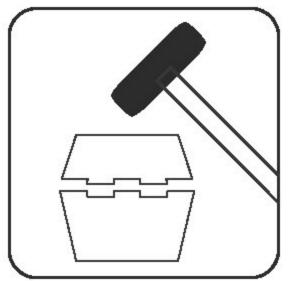
Press the parts together or use a hobby hammer with slight force for assembly.
