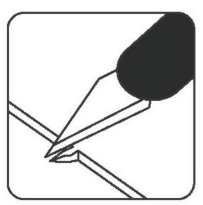
Use the exacto knife to remove any of the remaining connection bits.
