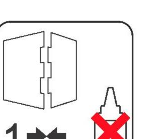
Always dry-fit the parts to together without any glue to make sure you are assembling the correct parts.
