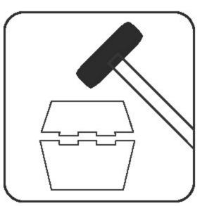
Press the parts together or use a hobby hammer with slight force for assembly.
