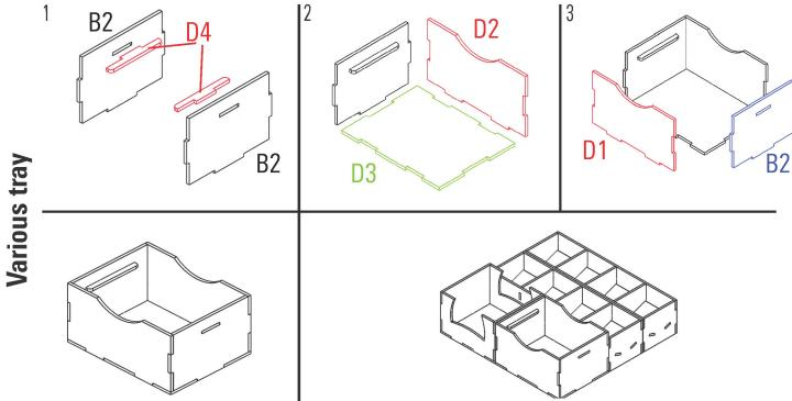
Required parts: **B2**x2,**D1,D2,D3 D4**x2
