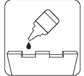
Use a drop of glue along the joints and hold it in place until the glue has sufficiently dried.
