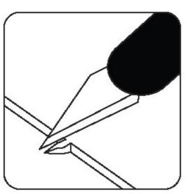
Use the exacto knife to remove any of the remaining connection bits.
