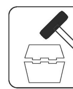
Press the parts together or use a hobby hammer with slight force for assembly.
