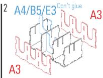
Required parts: **A1,A2**x2,**A3**x2,**A4**x4,**B5,C4**x2,**E3**
