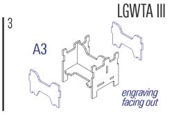
Required parts: **B7**, **D13**, **A16**x2, **A13**x2
