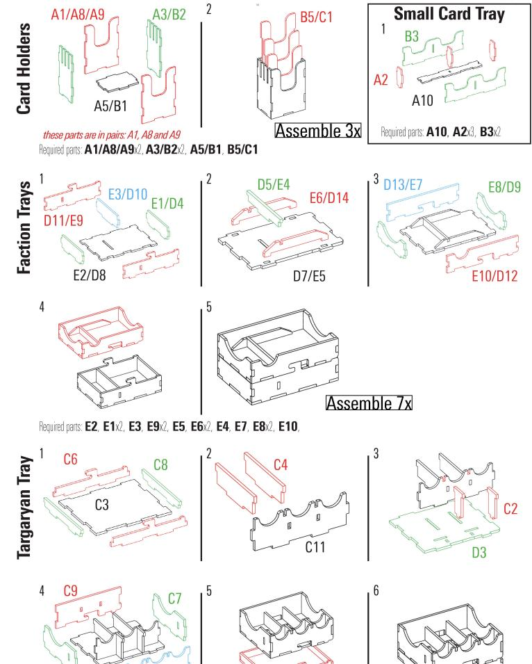
Required parts: C3, C8x2, C6x2, C4x2, C11, D3, C2x2, C10, C9, C7x2,
