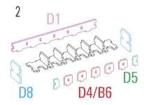
Required parts: **D9/B9**x5, **D2, D1, D8**x2, **D4/B6**x5
