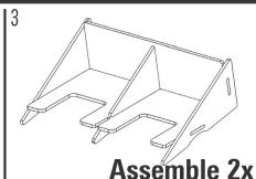
Required parts: **A5**x2,**A6**x2,**B6**x2,**B7**x2,**D1**x2
