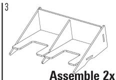
Required parts: **A5**x2,**A6**x2,**B6**x2,**B7**x2,**D1**x2
